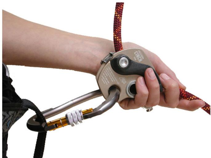
Correct technique for holding the Cinch. Use the right hand to feed rope. Note: hands can be switched.
